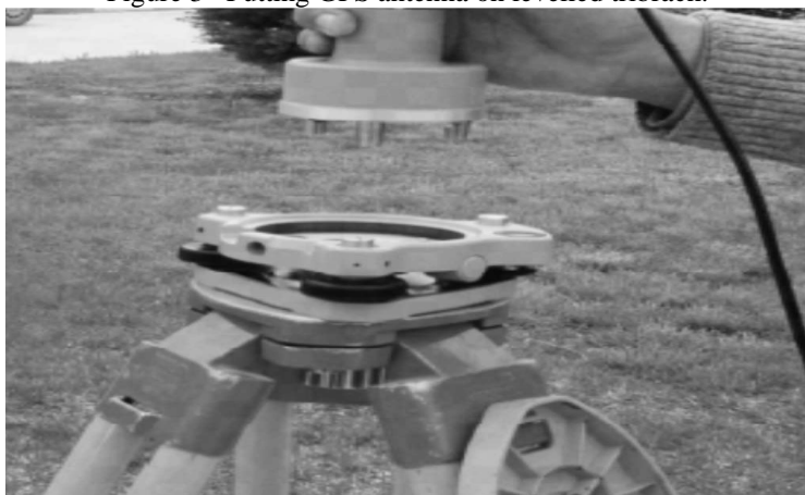
Figure 3 –Putting GPS antenna on levelled tribrach.
