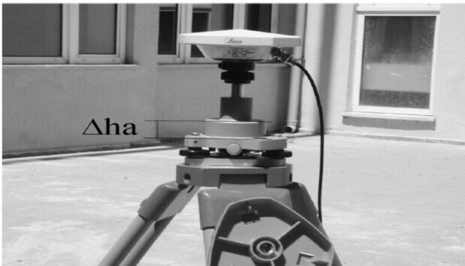
Figure 4 – Offset between GPS antenna reference point and reference surface of tribrach.
