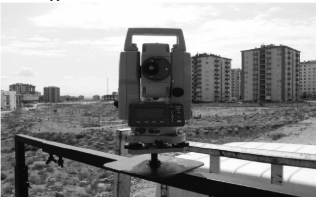
Figure 6 – The apparatus with attached total station used for detail survey.
