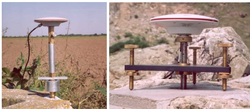
Figure 11-Antenna setup: CRC adapter (left), triangular plate (right).
