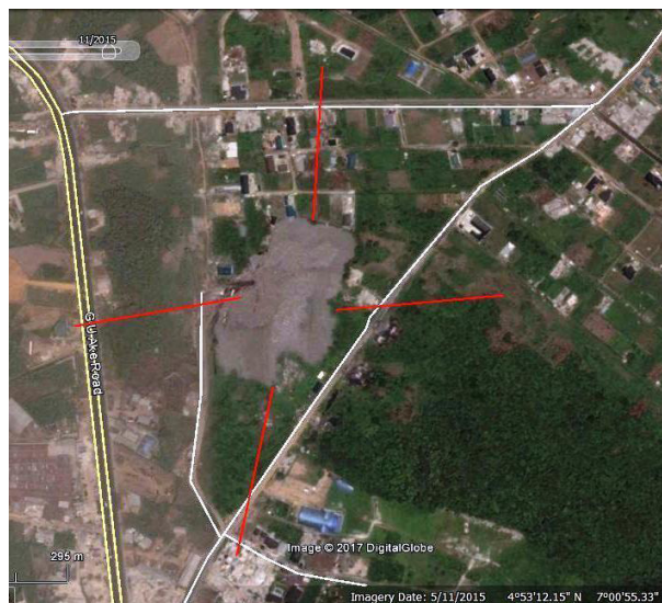
FIGURE 5 – Satellite image of Elioizu LFS planning area marked by red lines, which shows areas lying 250 metres from the edge of the landfills. SOURCE: adapted from Google Earth (2017)
