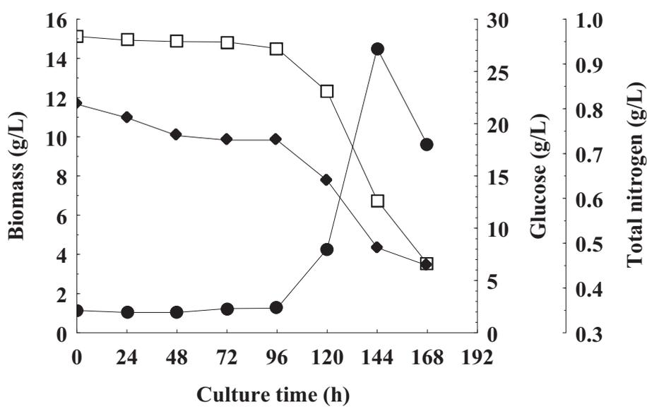
**FIGURE 2 - CONCENTRATIONS OF BIOMASS, GLUCOSE AND TOTAL NITROGEN DURING THE CULTIVATION OF *THRAUSTOCHYTRIUM* SP. ATCC 26185, USING 0.8 G/L OF TOTAL NITROGEN**
