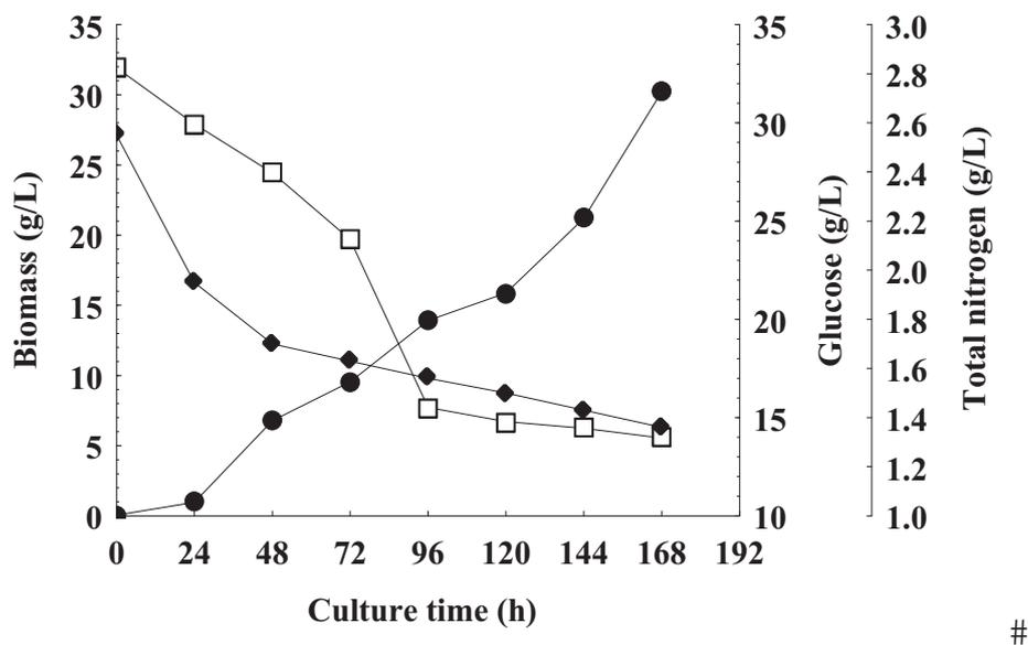
**FIGURE 1 - CONCENTRATIONS OF BIOMASS, GLUCOSE AND TOTAL NITROGEN DURING THE CULTIVATION OF *THRAUSTOCHYTRIUM* SP. ATCC 26185, USING 2.4 G/L OF TOTAL NITROGEN**
