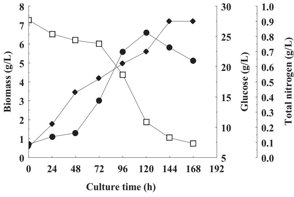
**FIGURE 3 - CONCENTRATIONS OF BIOMASS, GLUCOSE AND TOTAL NITROGEN DURING THE GROWING *THRAUSTOCHYTRIUM* SP. ATCC 26185, EMPLOYING FED-BATCH SYSTEMS 0.009 G/L (HOURLY) OF TOTAL NITROGEN**
